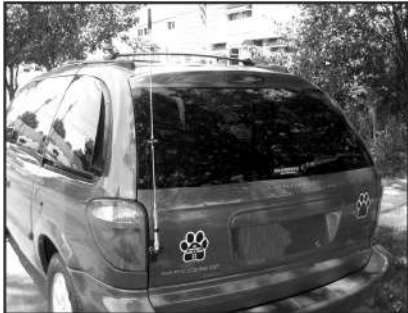
K400S mount with an NR790 (discontinued) Photo Courtesy: Joe Mitterando, KC2UZZ
